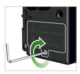
**4.** Put the battery compartment lid in correct position onto the gauge and fix it stress-free by the captive screw. When tight-ening, observe the maximum torque of 0.4 Nm.
